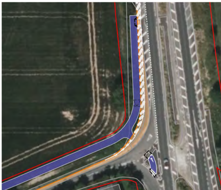
Figure 7.0 – A120 & Bentley Rd Junction widening and proposed cycle track layout (Option 3)
